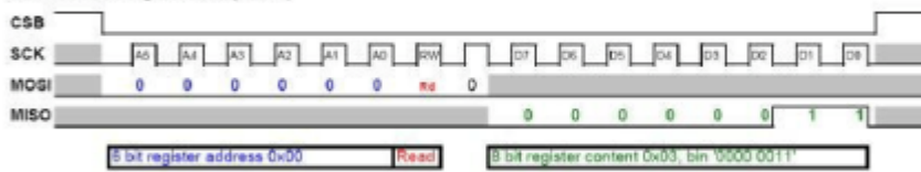
16 bit read from register 0x21 (TEMPOUT)
